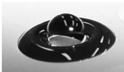
Fig. 6 A droplet splitter. The green water droplet sits on source and the red torus-shaped droplet on the target. These two droplets are separated by the ultrahydrophobic barrier. Nanostructured silicon surfaces for analytical applications
