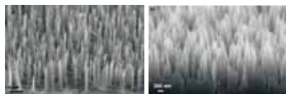
Fig. 3 Nanostructured silicon surfaces fabricated using a) silica nanoparticle mask combined with DRIE b) black silicon method.
