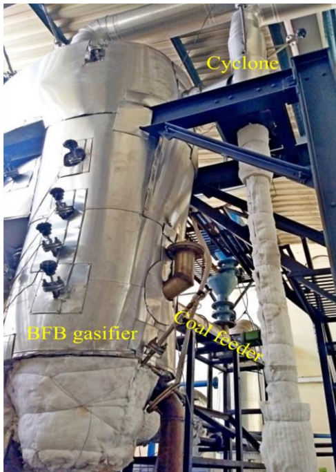
Figure #4: 300 kW th fluidized bed gasifier of high-ash coal: actual photograph (left), schematic diagram (right) (Gupta and De, 2022, Energy 244, 122868)
