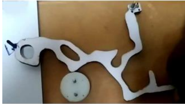
Figure #5: Synthesis of C^0 Path-Generating Contact-Aided Compliant Mechanisms Using the Material Mask Overlay Method. [Prabhat Kumar, et Al. 2016]
