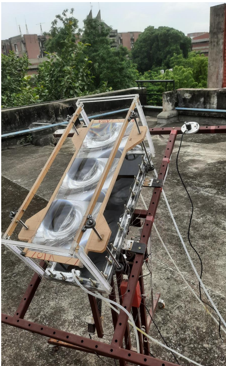
Figure #5: Solar desalination system based on Fresnel concentrators and nano-enhanced membrane
