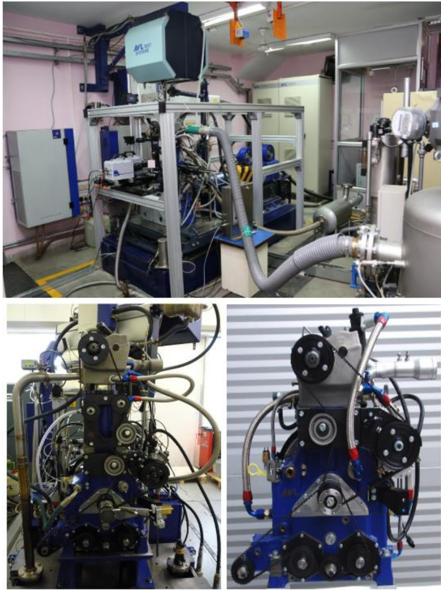
Figure #1: Single cylinder optical research engine (SCRE)
