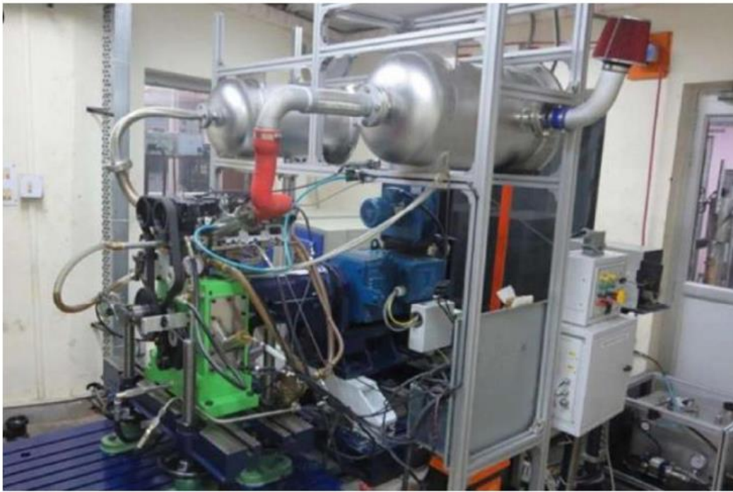
Figure #2: Experimental Setup of GDI Engine with the thermal head
