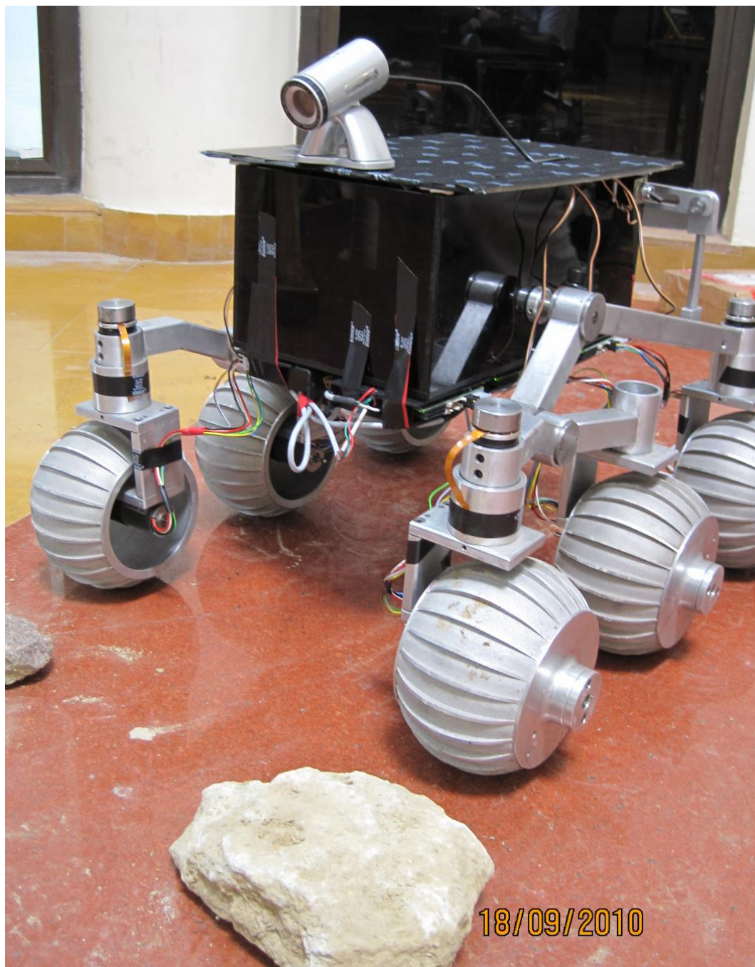
Figure #1: 14 DOF Lunar rover for space applications.
