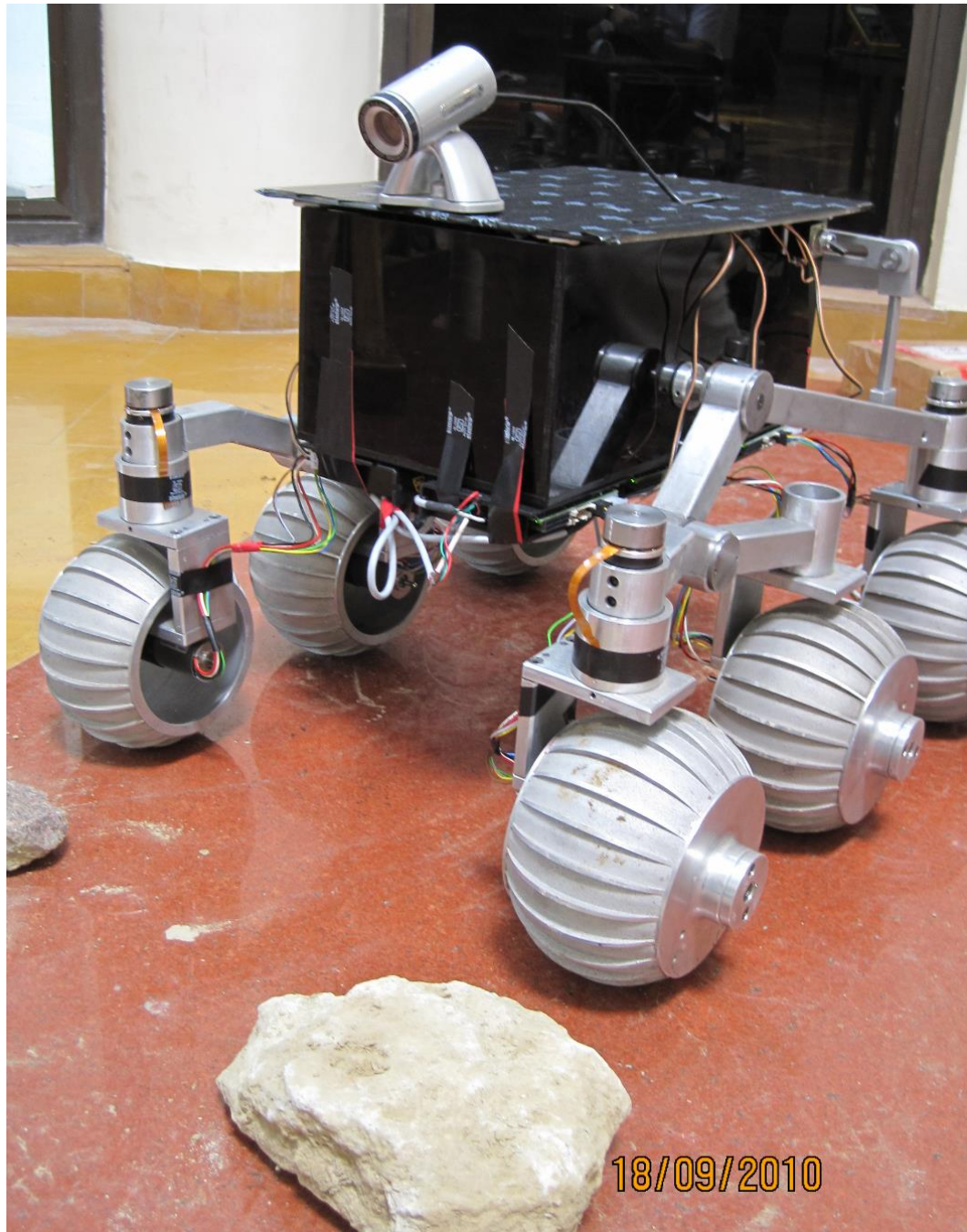
Figure #1: 14 DOF Lunar rover for space applications.
