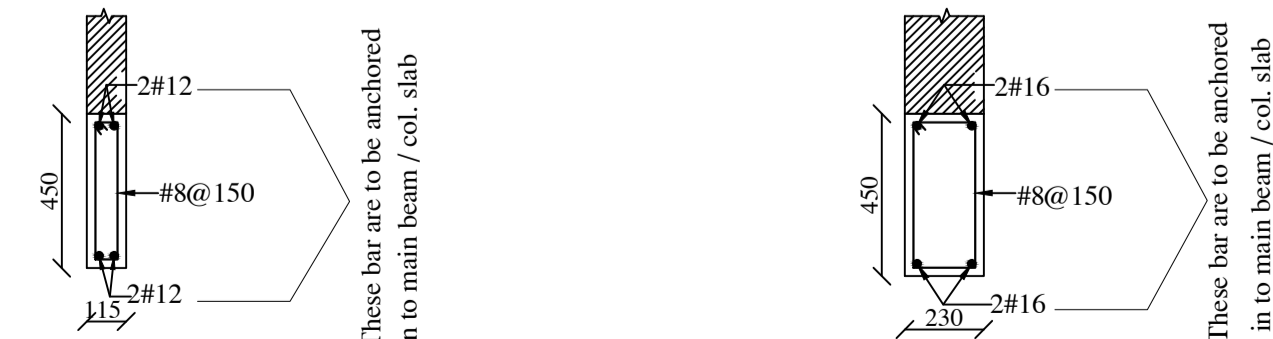
TYP. DETAIL OF RCC BAND (115X450) AROUND CUB BOARD / SHAFT / FINS TO SUPPORT 115 TH. BRICK WORK
