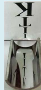
Nanofinishing of silicon (8 nm) by CMMRF process and stainless steel tube (16 nm) by R-MRAFF process
