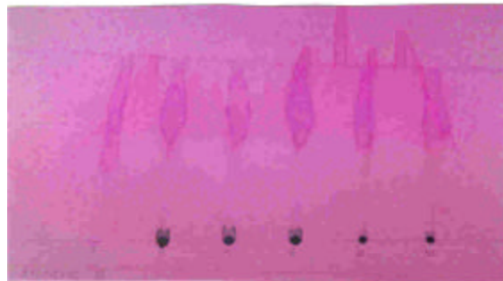
Figure 14: TLC of lubricating oils from diesel operated engine using Rhodamine-B revealing agent
