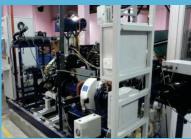
Two Cylinder Engine with Eddy Current Dynamometer
