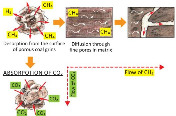
*A schematic illustration suggesting the micro-mechanisms and processes during CO<sub>2</sub> injection mediated enhanced CH<sub>4</sub> recovery. [Mukherjee & Misra, Earth Science Reviews, 2018]*
