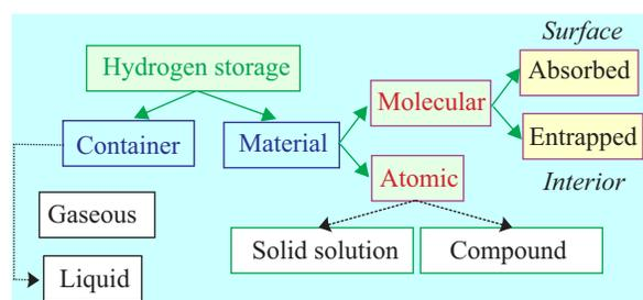
Figure 1: Multi-mode hydrogen storage philosophy to exploit storage of hydrogen in various phases
