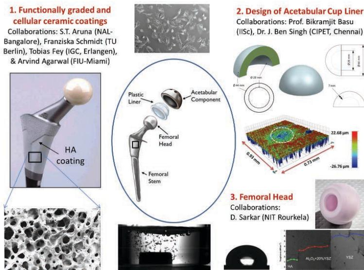
Fig. 1: Bird's eye view of the challenges associated with the design of hip-joint components (images from self-research & <https://www.molteno.com/m-sphere-natural-hydroxyapatite-orbital-implants> & [www.exac.com](http://www.exac.com)). These aspects are targeted in the current research.
