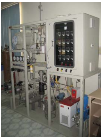
High temperature, high pressure bench-scale reactor for studies on monoliths and packed beds
