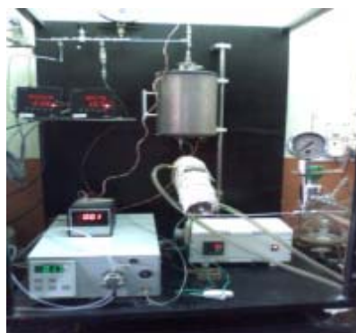
Set-up for in situ sulfiding of hydrotreating catalysts
