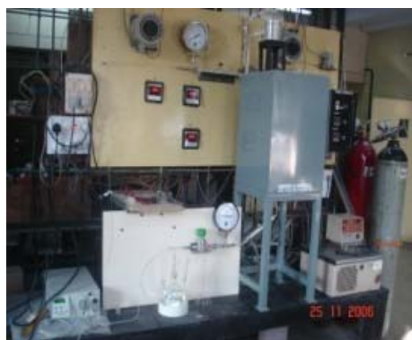
Monolith reactor for multiphase reactions
