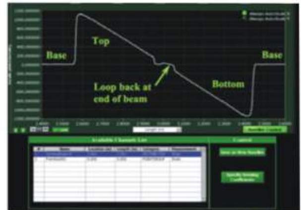
ODISI distributed strain measurement along the top & bottom surfaces of a cantilever beam, 5mm spatial resolution
