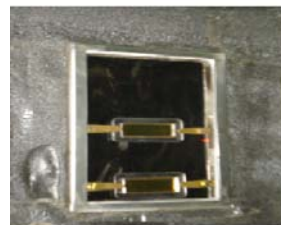
Zn-Se Window at the laser and detector ends of the fog chamber
