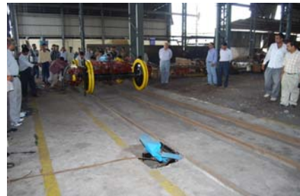
Derailment trial of Bogie using Derailment mechanism and brake actuator unit
