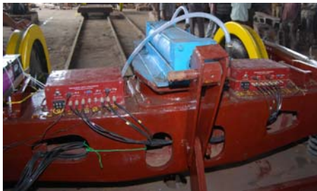
Derailment trial of Bogie using Derailment mechanism and brake actuator unit
