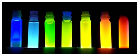
Figure 1. Luminescence emission from doped ZnS nanophosphors under UV excitation
