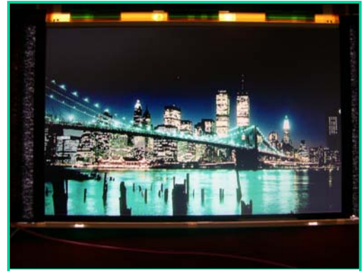
Figure 7 Working WVGA panel with integrated a-Si gate drivers
