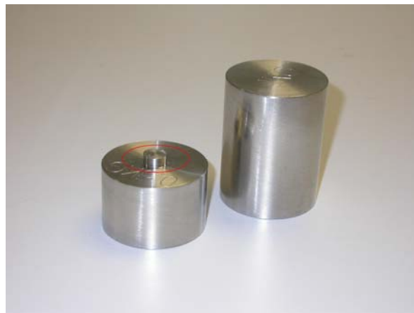
Figure 3. Photograph of counterweight.
